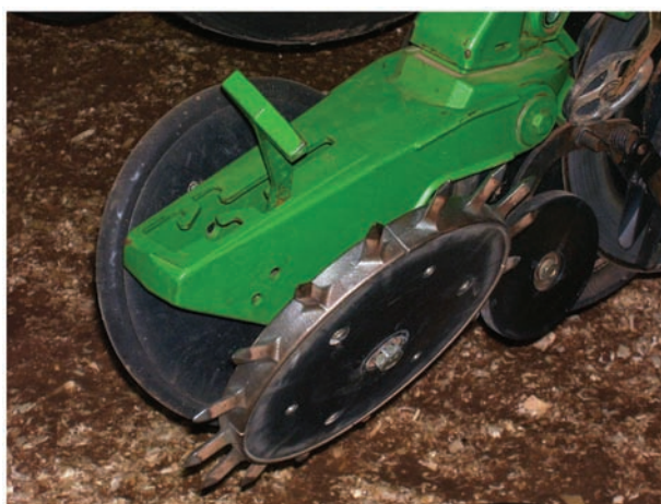
Figure 21. A spike closing wheel used with a standard John Deere closing wheel.
