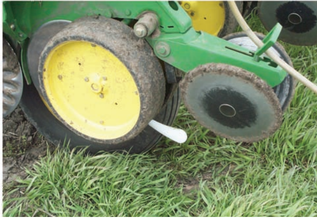
Figure 23. A Keaton seed firmer on a John Deere planter.
