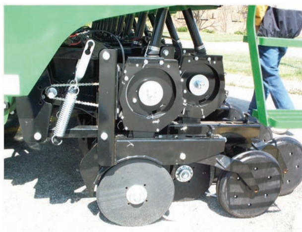
Figure 7. A Great Plains no-till drill with parallel linkage system.
