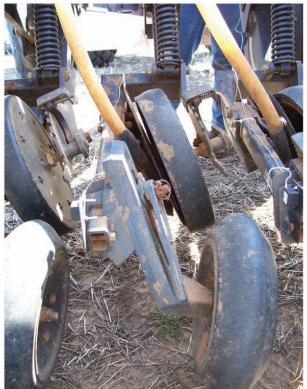
Figure 4. A single disk opener on a Flexi-Coil air seeder. Note the tilted opener disk.
