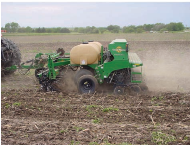
Figure 11. A Great Plains no-till drill operating in milo stubble.
