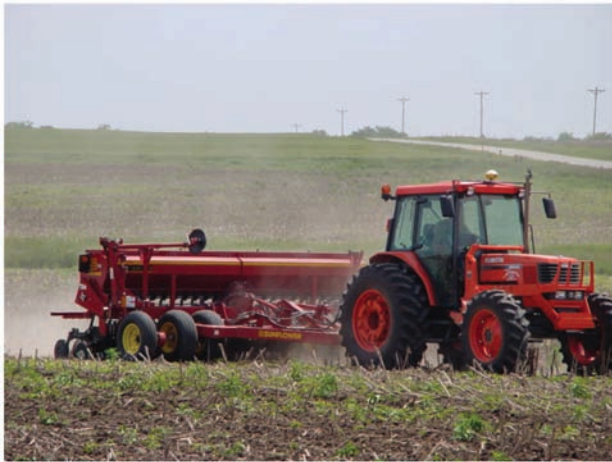
Figure 3. No-till drilling soybeans into milo stubble.
