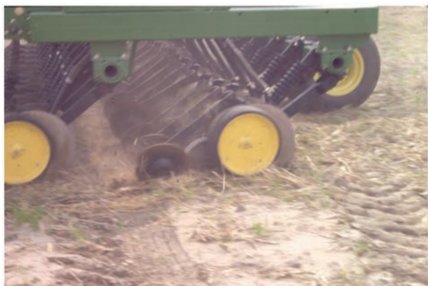
Figure 5. A single-disk opener operating in wheat stubble.
