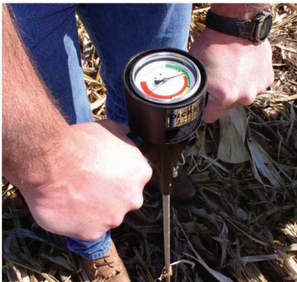
Figure 7. Using a density tester to locate compacted zones in soil.
