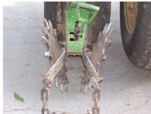
Figure 22. Spoked closing wheels on a John Deere planter.
